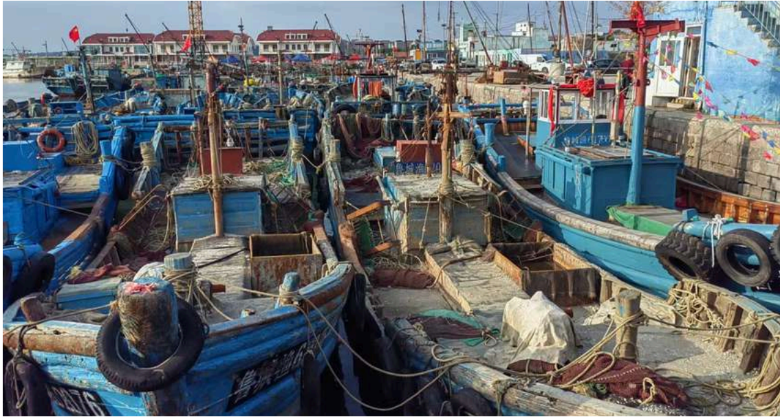
Figure 2: Clam fishing boats at Hong Dao China. Clam dredges can be seen either side of the superstructure on the left and centre boats. These polyvalent vessels harvest Manila clams scattered as juveniles for fattening over about 100,000 hectares of shallow seabed ranging about 5nm offshore. (Photograph: John Humphreys)
