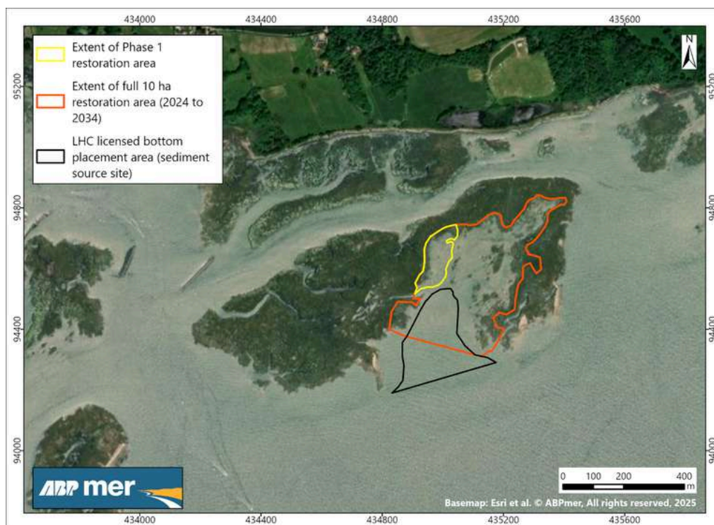
Phase 1: Map showing Boiler Marsh, Lymington Harbour. The orange line outlines the 10 ha ‘Beneficial Use of Dredged Sediment (BUDs)’ location which should be delivered within 10 years. The yellow line outline was the Phase 1 BUDs trial area and the black line shows the sediment source site, as in where the sediment was dredged from.
