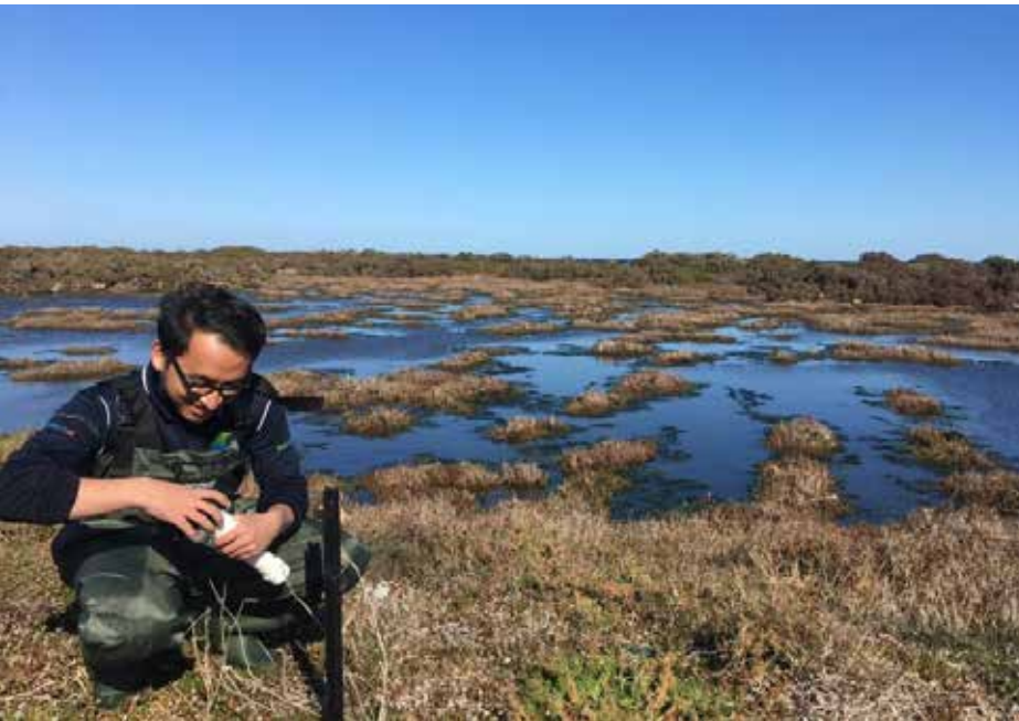
Figure 2 | Jaya deploying water level logger in coastal wetlands
