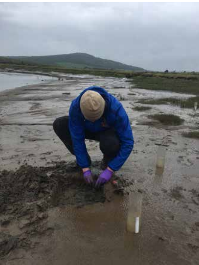
Wrapping a sediment core for geochemical analysis. Credit, Dr. Clementine Chiol.
